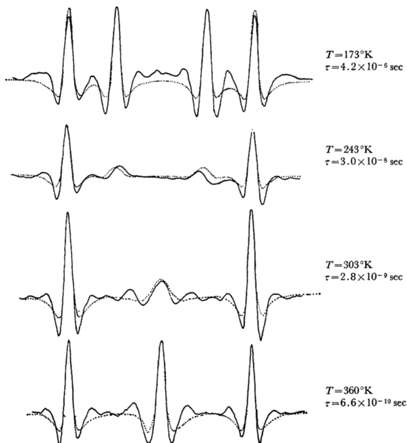
Fig. 5. Observed (solid lines) and calculated (dotted lines) second derivative ESR spectra of \text{CH}_2\text{COO}^- in the crystal for the magnetic field parallel to the c axis at different temperature T . The calculated spectra are obtained according to Eq. (2) together with Eq. (3) and the values of E and f_0 indicated in (4).
